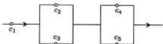
It is given that the components  $c_1, c_2, c_3, c_4$  and  $c_5$  have component reliabilities 0.6, 0.4, 0.7, 0.8 and 0.5 respectively.
