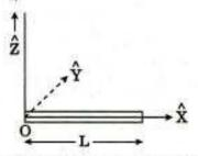
A rod of length L has non-uniform linear mass density (mass per unit length)  $\lambda$ , which varies as  $\lambda = \lambda_0 \left(\frac{S}{L}\right)$ ; where  $\lambda_0$  is a constant and S is the distance from the end marked 'O' (as shown in the figure). Find the centre of mass of the rod.
