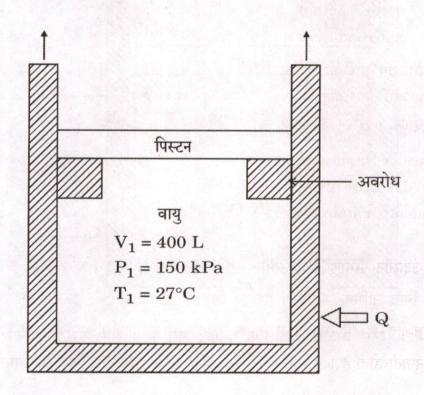
A piston-cylinder device initially contains air at 150 kPa and 27°C. At this state, the piston is resting on a pair of stops, as shown in the figure, and the enclosed volume is 400 L. The mass of the piston is such that a 350 kPa pressure is required to move it. The air is now heated until the volume is doubled. Determine:
