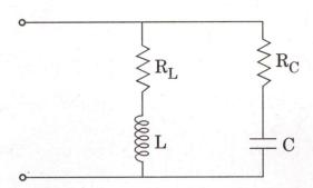
Consider the two branch parallel circuit shown in the diagram.
