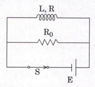
In the given circuit,  $L=2.0~\mu H$ ,  $R=1.0~\Omega$ ,  $R_0=2.0~\Omega$  and E=3.0~V. Find the amount of heat generated in the coil after the switch S is disconnected. The internal resistance of the source is negligible.
