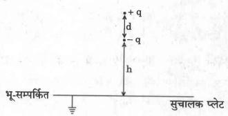
A vertically oriented electric dipole having dipole moment  $\overrightarrow{p}$  is kept at height h above an infinitely large horizontal conducting plate, which is grounded as shown in the diagram. Calculate the force between the electric dipole and the conducting plate by using method of images.
