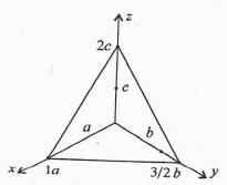
A crystal plane is shown in the above figure. Find its Miller indices and interplanar spacing.
