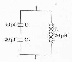
Explain how the circuit shown above can be a source of oscillations. Use this circuit to construct a transistor oscillator and explain its working. What is the frequency of oscillations of this circuit?
