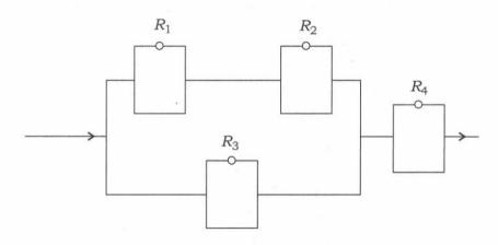
Define series system and parallel system. In a system, four independently and identically distributed components are connected as per the following configuration. Each component has exponential lifetime with mean equal to 200 hours. Obtain system reliability at time 300 hours :
